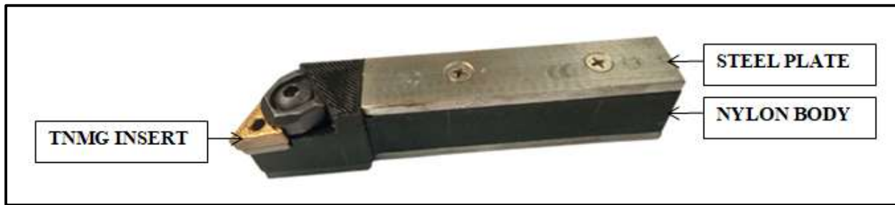
Fig. 1 FFF 3D Printed Flitched Tool holder for TNMG Insert
