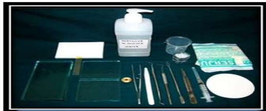
PHOTOGRAPH III : ARMAMENTARIUM USED FOR MAKING CEMENT SPECIMENS
