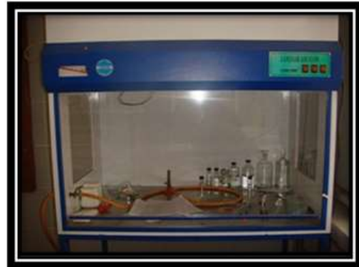
PHOTOGRAPH VIII : LAMINAR AIR FLOW UNIT
