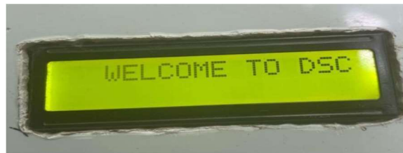
Fig 10: Status when power switch is turned on.
