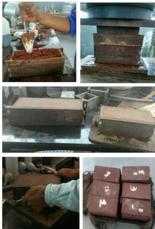
Fig 1 Process of Casting of Cement stabilized masonry blocks
